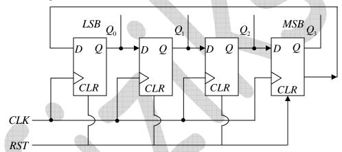
the binary number given by the string  $Q_3, Q_2, Q_1Q_0$  changes for every clock pulse that is applied to the CLK input. If the output is initialized at 0000, the the corresponding sequence of decimal numbers that repeats itself, is
